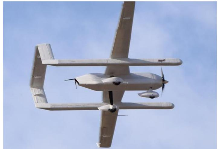
Northrop LHO vehicle has quad rotors for vertical take-off & landing (VTOL) with a quiet cruise tractor propeller for fixed wing flight. The 386 cubic inch internal payload bay is in the rear of the center fuselage over the wing.
