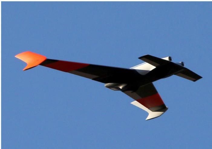
Boeing LHO vehicle has an internal electrically driven ducted fan on the right side of the fuselage with an inlet & exhaust duct. Adjacent to the fan is a 400 cubic inch internal payload bay between the wing and canard.
