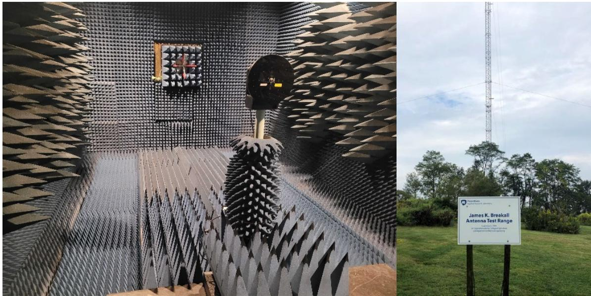
Anechoic chamber (left) and 40 m tower at the outdoor antenna test range control room (right)
