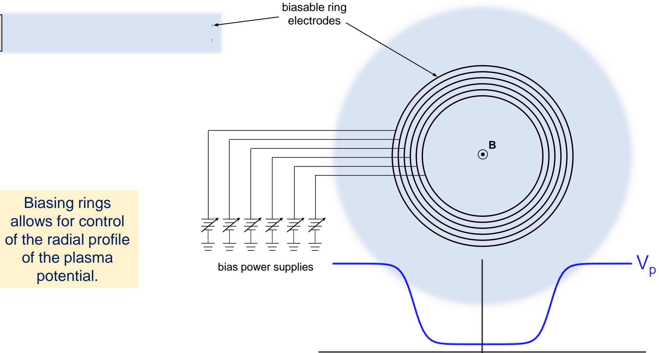
Biassing rings allows for control of the radial profile of the plasma potential.
