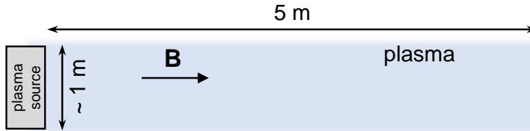
The NRL Space Chamber plasma is  $\sim 1\text{-m dia} \times 5\text{-m long}$ , surrounded by  $\sim 0.5\text{-m}$  vacuum gap to minimize boundary effects.
