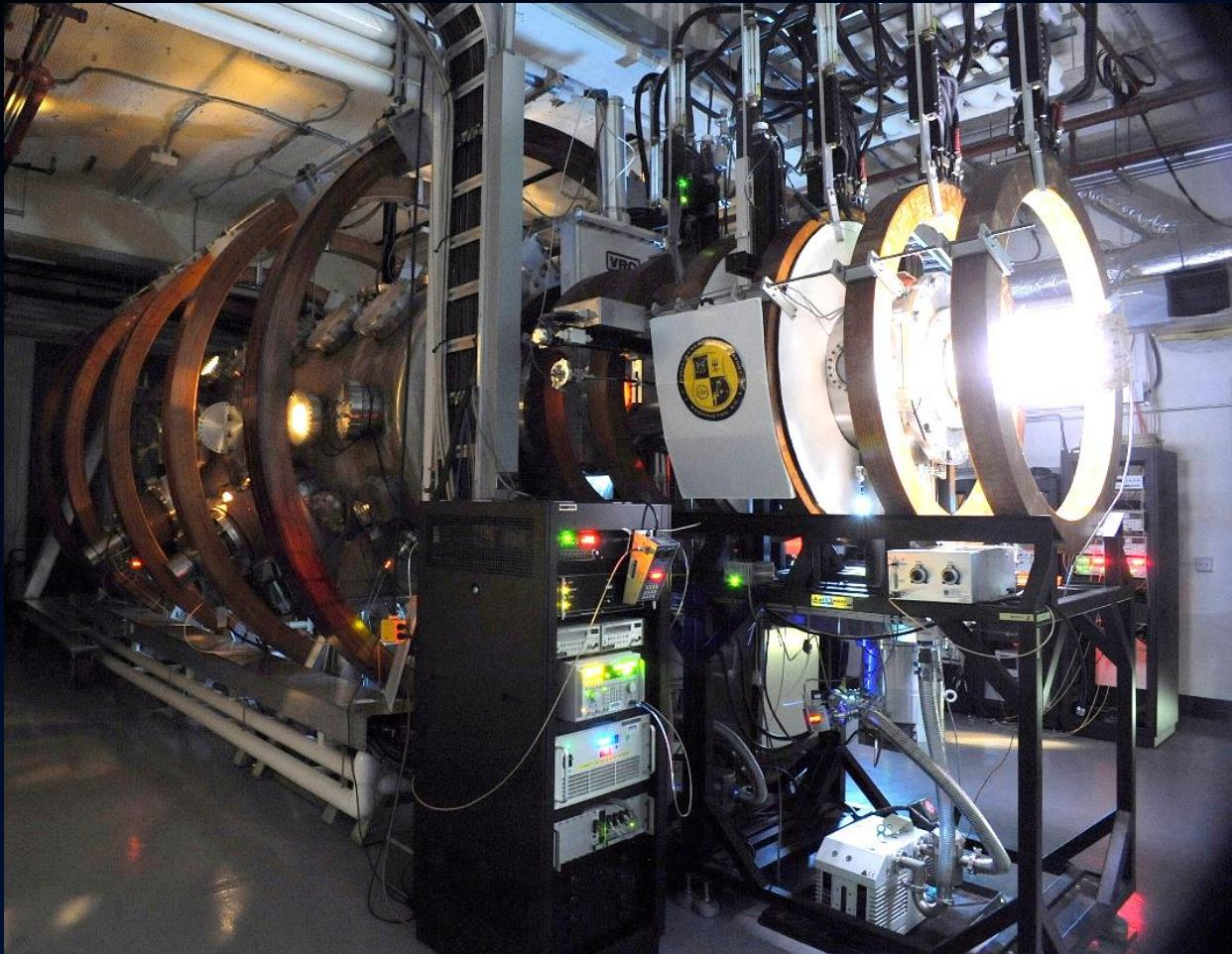
NRL Space Physics Simulation Chamber (SPSC). Scaled near-Earth space-like plasmas are created in the SPSC's 5-m long by 1.8-m diameter main chamber and 2-m long by 0.55-m diameter source chamber. Independently controllable electromagnets allow for control of the shape of the axial magnetic field.
