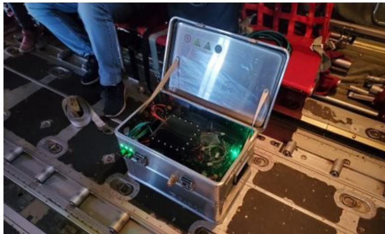
Photograph of the ACHILLES chemical sensor developed by SRI International during decontamination flight testing on a C-130J Air Force cargo plane.
